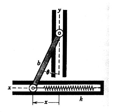
2. For the slide-crank configuration shown below, derive the expression for the velocity  $v_A$  of the piston (taken positive to the right) as a function of  $\theta$ . (20%)
