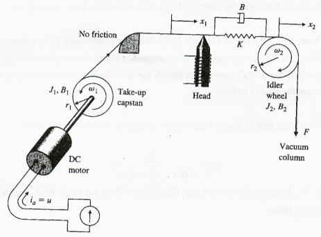
(1) (20%) Write the equations of motion in terms of the parameters listed below. K and B represent the spring constant and the damping of tape stretch, respectively, and  $\omega_1$  and  $\omega_2$  are angular velocities.
